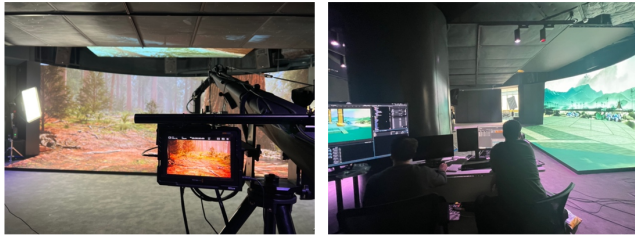
Figure 2: Showcases 3D virtual sets displayed on an LED video wall and used for live compositing with 4K moving cameras.
