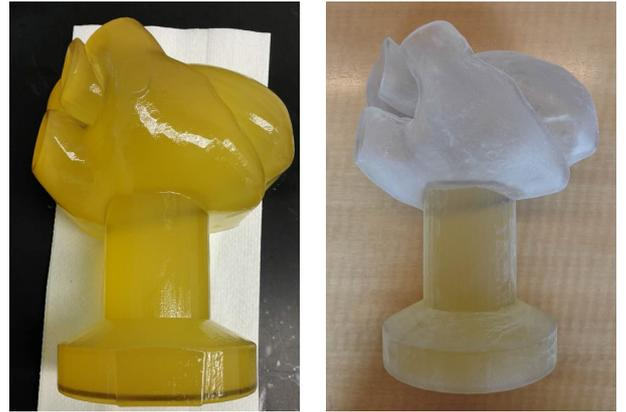
Fig. 2. Newly printed object (left) and after post-processing, which is used as the pre-existing model.
